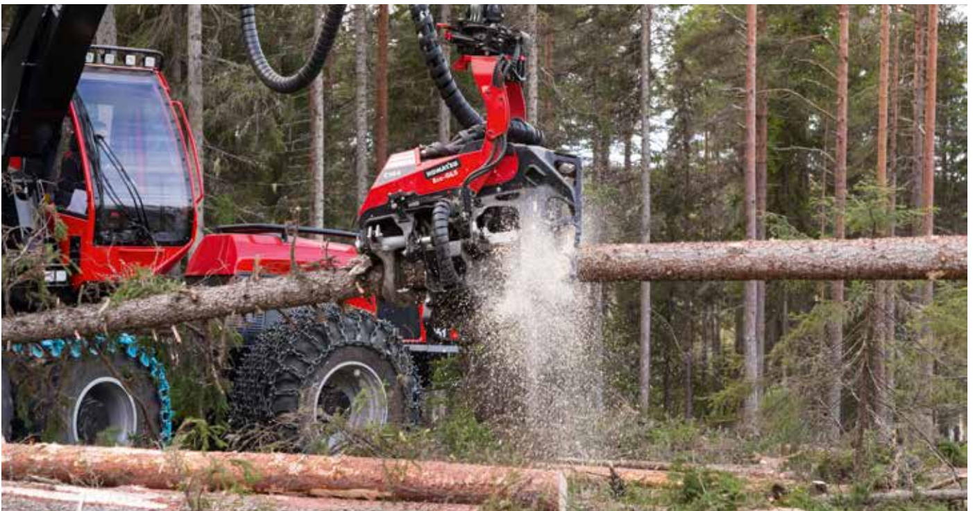
An Eco-GLS greased chain reduces environmental impact. Available as an option for the Komatsu C93, C123, C124, and C144 heads.
