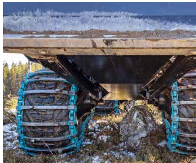
Portal bogies ensure the best possible ground clearance for forwarders and harvesters alike.
